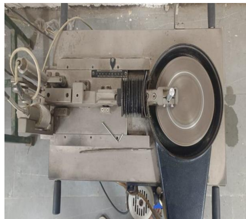
e) Top view of pin-on-disc setup
