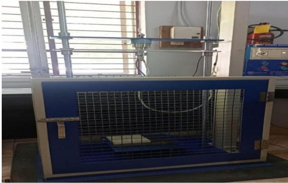
Fig. 1. Experimental drop-weight impact test machine used for the sandwich specimens.
