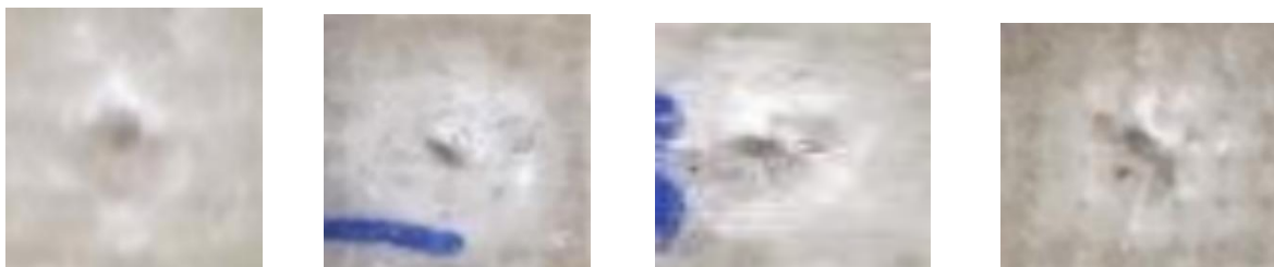
Fig. 4: c) Impact Damages after Failure of the Specimens in Different Loading Conditions.
