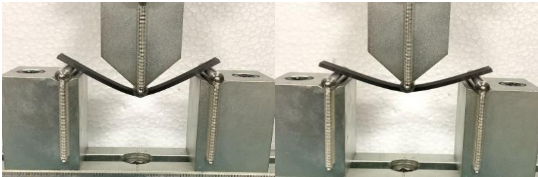
Fig.4. Samples before and after relaxing (left) and their maximum bending (right)
