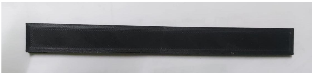
Fig.2. Printed Specimen for flexural test of Iron-PLA material.
