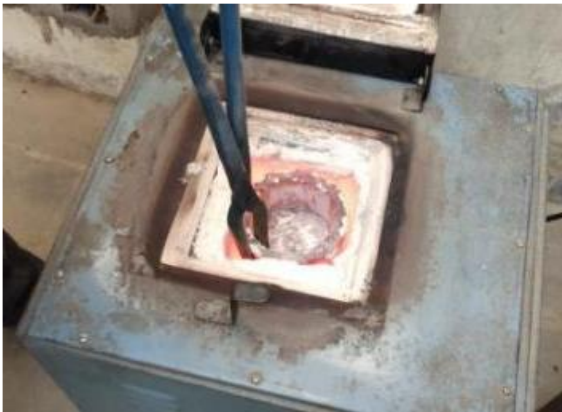
Figure 2. Al 7075 furnace activity to remove the impurities
