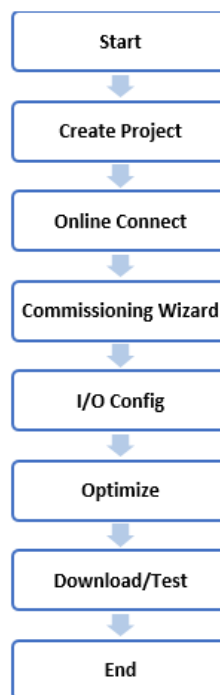
Fig. 4 Configuration of SINAMICS G120 using software TIA Portal
